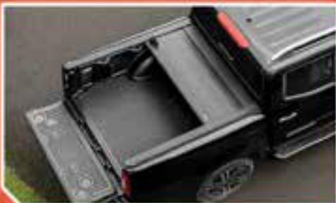
The TRUCKMAN Retrax retractable tonneau cover is constructed from industrial strength aluminum slats that provide supreme strength and ruggedness, as well as heavy-duty matte finish.
