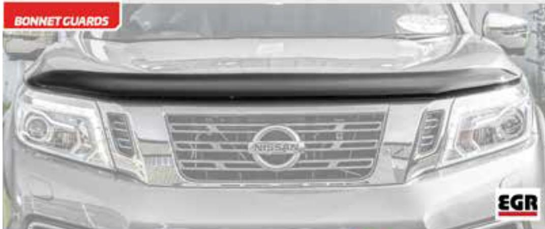
Bonnet guards provide maximum protection for your bonnet paintwork from stone chips. Our guard range from EGR is individually designed to follow the contours of each vehicle.
