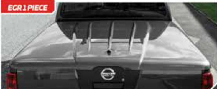
A single point push button locking system is used along with gas struts to assist opening and closing.
